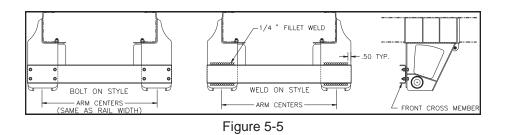
CAUTION: Crossmember must be installed for proper and safe suspension operation.
