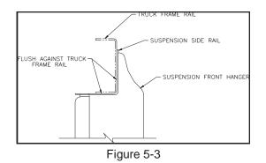
8. Mark the location of the mounting holes on the outward side of both Auxiliary Suspension Frame Rails.
