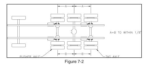
4. <u>IMPORTANT:</u> Recheck alignment, then weld 1/4" minimum fillet weld allaround alignment collars to hanger side plate. (total of four collars)
