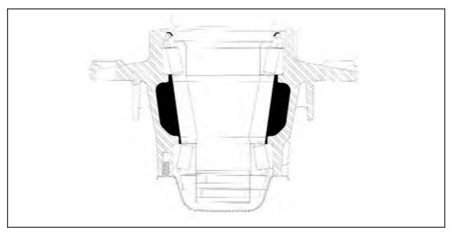
Fig. 6: Lubrication Fill Greases (Nos. 1,2, & 3)
