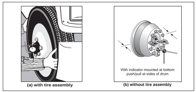
Fig. 1: Dial Indicator Set-Up
