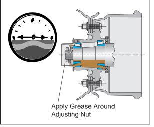
Fig 5A: Lubrication Fill Semi-Fluid Grease (No. 00)
