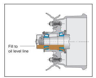
Fig. 3: Lubrication Fill Oil (Static)
