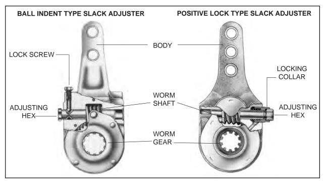
Fig. 1: Manual Brake Adjusters
