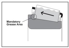
Fig. 4: Packing of Bearing Cone
