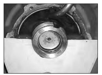
Fig. 5: Semi-Fluid Grease Top Off Procedure
