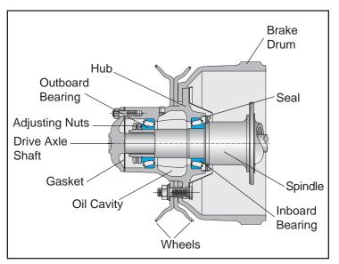
Fig. 2: Drive Axle Wheel End
