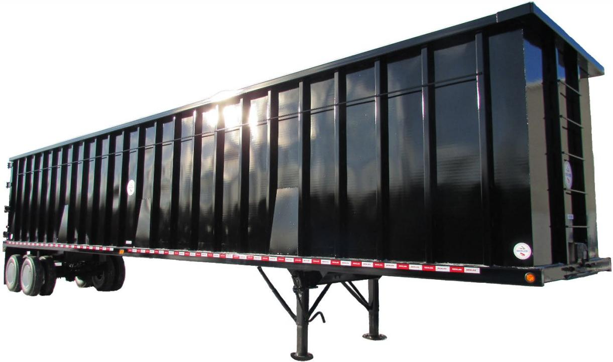
BENLEE manufactures and sells the best Open Top Gondola scrap trailer in the market, with the lowest owning and operating cost. They are mostly sold in 48' and 53' lengths with 8' high sides, made from Hardox, thin, high strength steel to carry the most possible weight, which lowers your transportation costs. Call us for a quote.
