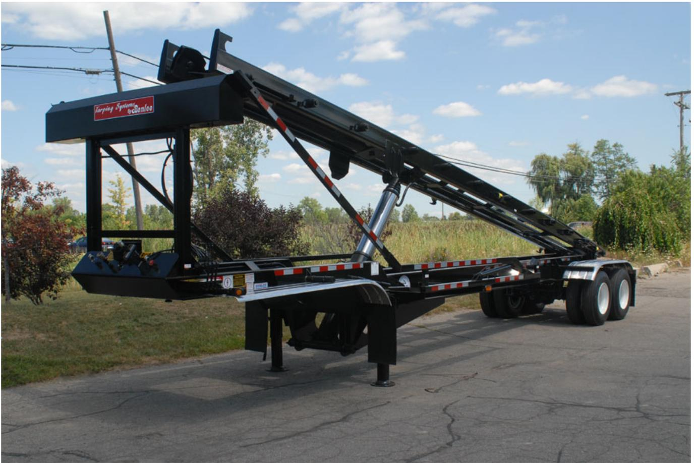
Product of the week is BENEE's BridgeMaster. This redesigned 80,000 GVW trailer weighs almost 9,000 pound less than the standard conventional trailer, so it can carry almost 20 percent more weight than a Conventional tri axle trailer.
