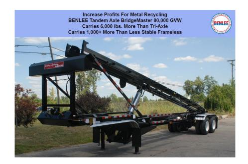
Lowering transportation costs is one of the keys to increased profits in Metal Recycling. BENLEE's 80,000 lb. GVW 40' Tandem Axle Bridge Master carries 6,000 lbs. more than our Triaxle conventional trailer. Also due to the BridgeMaster has a longer wheelbase bridge, than a less stable frameless 40' trailer, the BENLEE carries more weight, not less weight than a Frameless 40' trailer with a normal the common wheelbase Tractor. Call us for a quote.
