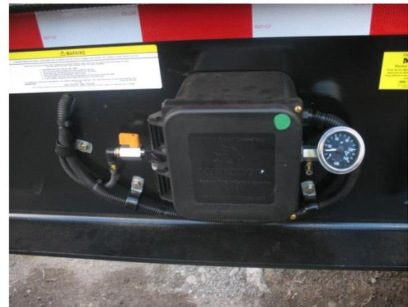
Options available on our trailers include: Air inflation system (picture above), grease systems, filtration system, aluminum rims, tarps, inside cab controls, tool boxes, stinger tails, aluminum fenders,
